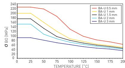
$\sigma_{Bo}$  diagrams represent  $\sigma_{Bo}$  values for different gasket material thicknesses. These values indicate the maximum in-service compressive pressures which can be applied on the gasket area involved without destructing or damaging the gasket material.
